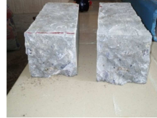
a: unreinforced cement composite beam (control).
