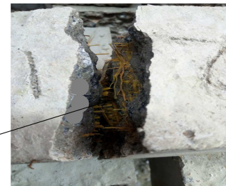
b: 1-fabric layer reinforced cement composite beam.
